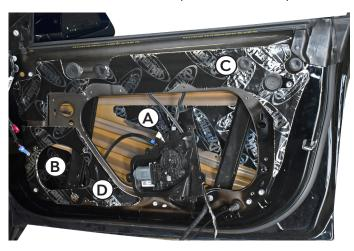
Tip: Partially pre-peeling release paper backing and folding aluminum faces together makes this easier. Adhere to door. Smooth with Dynamat roller for best results.
