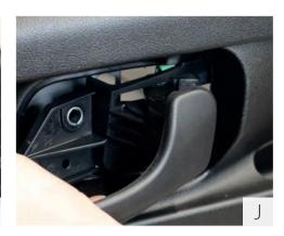
D: Use your finger to pry out the door handle connection and remove the door handle. (Fig. I)
