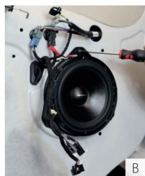
• Disassemble all screws of the factory woofer (pick up screws) 3x TX20
