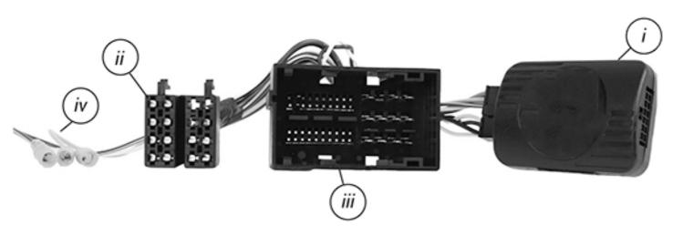
i. Interface Box ii. Male ISO Connector (16 Pin) iii. Fiat Vehicle Connector iv. Flying Wires (Green - Park Brake / Pink - Speed Pulse / Purple/White - Reverse Gear)
