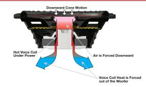
As Cone Moves Downward, the Hot Air is Forced out of the Woofer. When the Cone Moves up, it Draws in Cool Outside Air.
