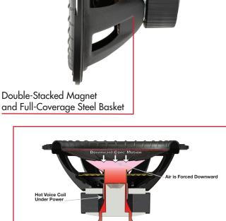
Voice Coil Heat is Forced out of the Woofer As Cone Moves Downward, the Hot Air is Forced out of the Woofer. When the Cone Moves up, it Draws in Cool Outside Air.
