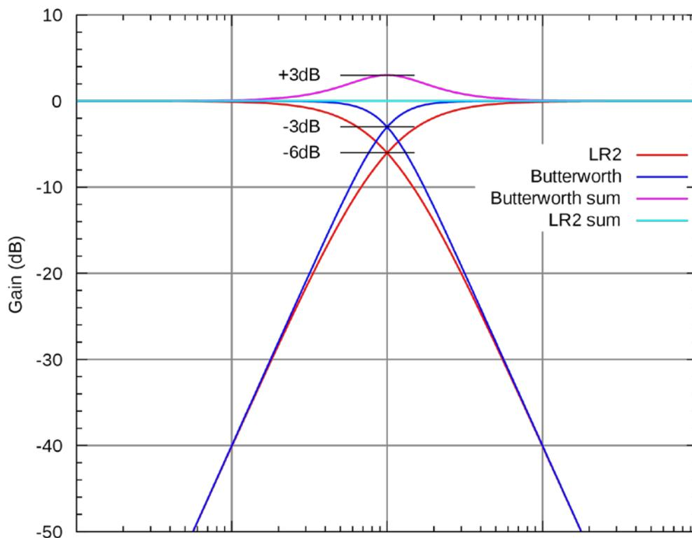
sum together at the crossover point. Electronically speaking, a Linkwitz-Riley implementation sums together to a flat response at the crossover point and a Butterworth implementation sums with a +3dB rise at the crossover point. However, in a vehicle, drivers could be located almost anywhere, so perfect driver physical alignment and control of acoustic interaction may not be possible, so all bets are off. The best
