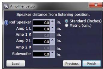
Set the distance of each speaker from the primary listening position. This will automatically configure the correct time-delay for each speaker to present the best sound-stage. The Reference Speaker setting should be set if there is a speaker in use that is not connected to your currently chosen amp, and is also the farthest from the listening position.
