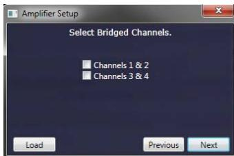
Choose to bridge the channels if both channels are used to drive a common load.
