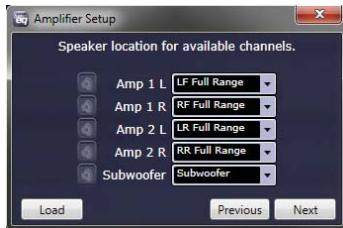
Select the type of driver used by each channel. This will assist the TWEEQ software in automatically configuring your crossover. See Page 13 for reference chart.
