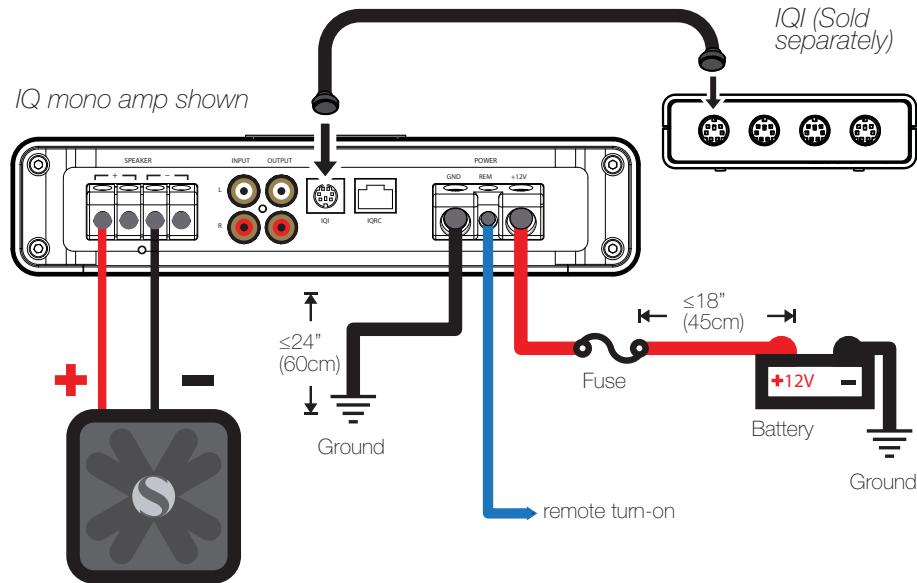
Wire your speakers to the IQ amplifier using 16GA or larger wiring. Connect the output of your source unit to the RCA Inputs of the IQ amplifier. Use the IQ's RCA Outputs to pass the signal to another amplifier.
