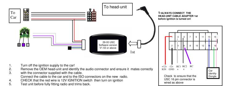
If Problems: Check that correct adapter has been used and links are in the correct place. Always disconnect from the power supply if you change the head-unit adapter lead. Check that Red wire is 12V ignition and not Permanent power. Check that head-unit is earthed and black wire is earth. Check all connections are the same as the wiring diagram shown here. If using PS-PCB software version (written on control box) must be 1.95 or higher. If not ASCPIO3V must be used.
