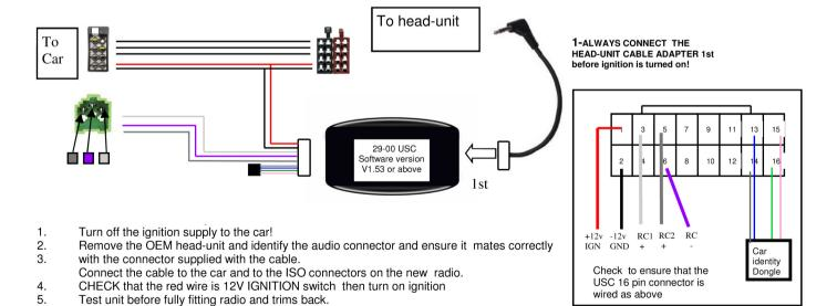
If Problems: Check that correct adapter has been used and links are in the correct place. Always disconnect from the power supply if you change the head-unit adapter lead. Check that Red wire is 12V ignition and not Permanent power. Check that head-unit is earthed and black wire is earth. Check all connections are the same as the wiring diagram shown here. If using PS-PCB software version (written on control box) must be 1.95 or higher. If not ASCPIO3V must be used.
