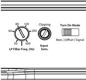
To properly set the amplifier for maximum clean output, please refer to Appendix A (page 12) in this manual. After using this procedure, you can then adjust the “**Input Sens.**” levels downward if this is required to achieve the desired system balance.
