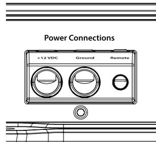
The amplifier's "4+12 VDC" and "Ground" connections are designed to accept up to 4 AWG copper power wire.
