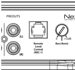
The RBC-1 connects to the jack labeled “**Remote Level Control (RBC-1)**” on the Connection Panel of the amplifier using a standard telephone cable (supplied with the RBC-1). If desired, multiple JD monoblock amplifiers can be controlled from a single RBC-1 controller using a single-line, four-wire phone line splitter and multiple phone cables.
