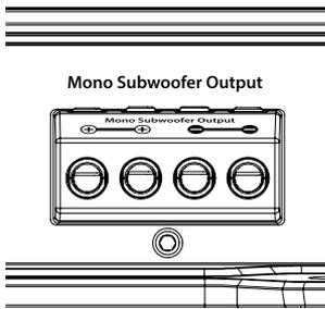
You will notice that there are two “+” positive connections and two “-” negative connections. This is to facilitate multiple subwoofer wiring.
