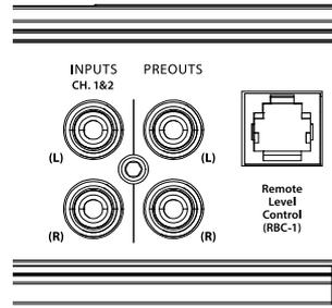
**Note:** The preamp output signal is not affected by the amplifier’s filter controls. If the input signal is full-range, the preamp output will be full-range.
